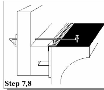
**Step 7.** Drive the concrete nails into the bond beam 14" apart and 8" from the tile.
