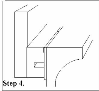
**Step 4. (Face Form)** Peel the paper from the double-faced tape (one foot at a time). Then line the bottom of the face form up with the bottom of the extender. Stick the face form to the extender.
