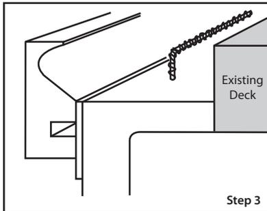
**Step 3.** Peel the paper from the double-faced tape one foot at a time, sticking the form to the tile with the lower edge of the form profile, even with the top of the tile.
