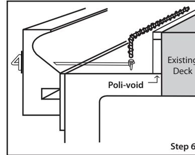
**Step 6.** Apply spray adhesive to the existing deck. Let stand 1 minute. With the perforated tear strip up, press the Poli-Void level to the existing deck.
