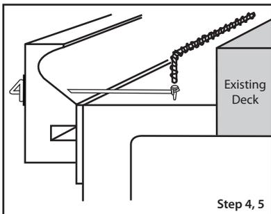
**Step 5.** Place the plastic washer (provided) on the tie wire. Push the tie wire through the form, even with the top of the tile. Wrap the end of the tie wire around the concrete nail, applying slight pressure.
