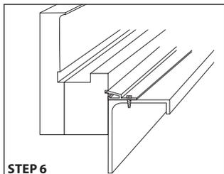
**STEP 6.** Peel the paper from the double-faced tape on the face form 1 foot at a time. Line the bottom of the face form up with the bottom of the extender. Press the face form to the extender.
