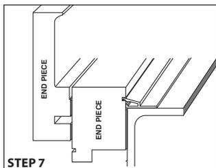
**STEP 7.** The end pieces should be set on the end of the pool, opposite of the roller. Place the extender marked "END PIECE", on the pool wall upside down.
